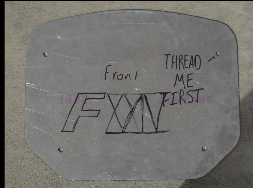
Anti-Intrusion plate showing which fastener to thread first
