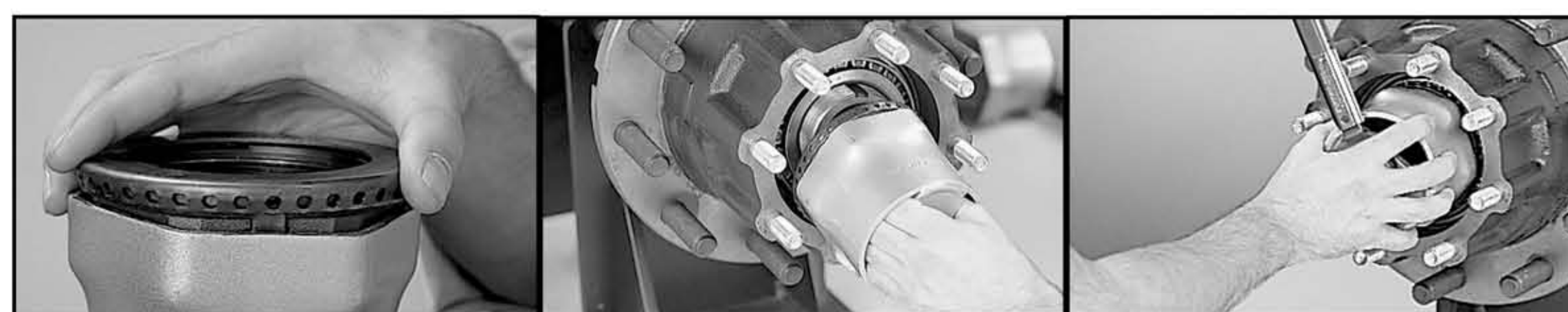
Figure 4. Place Axilok in correct size socket and check for free rotation.
