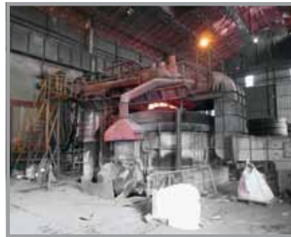
Preparation of the molten metal, e.g. in a 50-ton furnace. The tem- perature is measured through the slag opening. The casting temperature is reached at 1650 °C.
