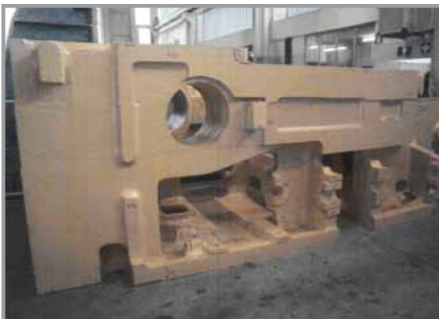
The cast now has to rest for two weeks in the earth until it has cooled down.
