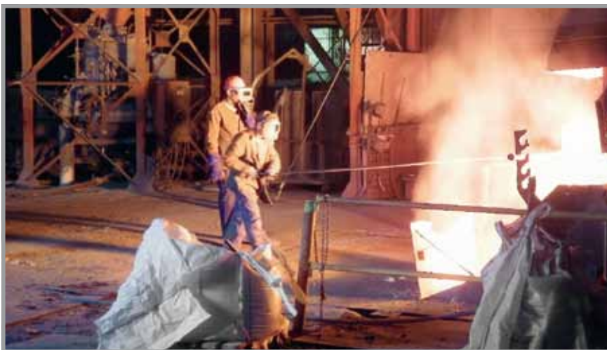
Slag is drawn off several times. The material sample from the furnace is immediately examined using spec- tral analysis, before the material is emptied into the casting ladle. The next material sample is taken from the casting ladle. The molten metal is only released for pouring if the material samples are judged acceptable in the inspection.
