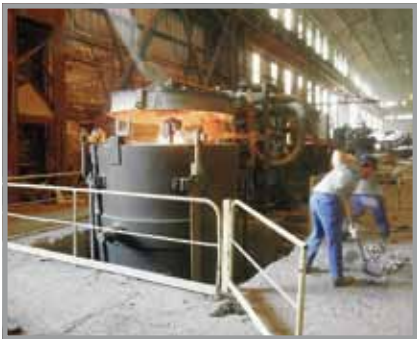
The casting ladles are prepared and heated up.
